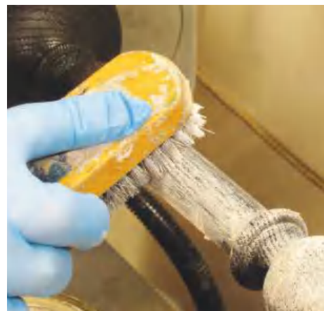
▲ Pic.33 Spray the work with ebonising lacquer and then apply the liming wax. The wax should be liberally spread all over the surface, paying particular attention to working it into the grain
